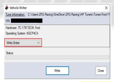
Once complete, you will need to turn the key off (wait 3 seconds) and then back on. Please note if you receive a Data Integrity "Check Failed" error message, that can be ignored. HP Tuners is aware of the error, but it has no bearing on the tune files you've loaded.
