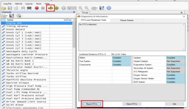
No DTC's were detected. However, if one or more DTC's are detected, please be sure to notate them during your data log submission. If you're instructed to clear the DTC codes. Please do so by clicking the "Clear DTC's" button.
