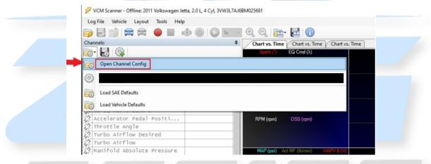
It is recommended that you connect to vehicle before starting a data log. This is done by plugging your RTD Flasher into the OBD2 Port of your vehicle and connecting your Laptop/Tablet to the RTD Flasher with the HP Tuners Supplied USB Cable.
