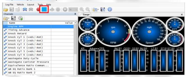
You will need to save the log file, to do so press Log File> Save Log As. Please include the tune type, the rev number, and a brief description in the name. Ex E50 Rev01-3<sup>rd</sup> Gear Pull
