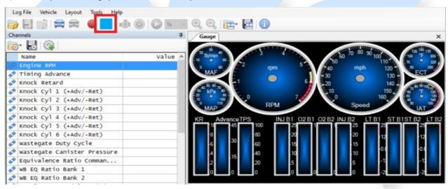
3) You will need to save the log file, to do so press Log File> Save Log As. Please include the tune type, the rev number, and a brief description in the name. Ex E50 Rev01-3<sup>rd</sup> Gear Pull
